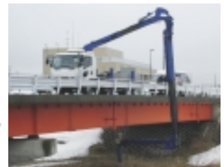
新型橋梁点検車「橋竜」 "Bridge Dragon" new model bridge inspection vehicle
