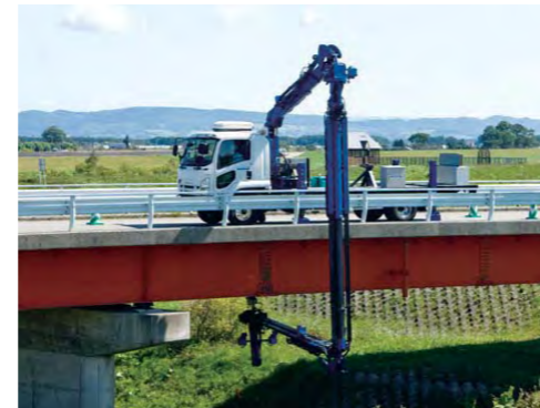
カナモトオリジナル設計の高性能遠隔橋梁点検車「橋竜」 Kanamoto's original design high-performance remote-controlled "Bridge Dragon" bridge inspection vehicle
