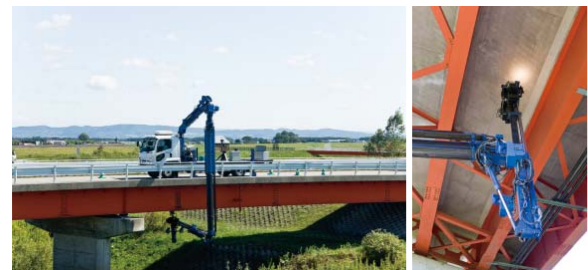
当社の橋梁点検車「橋竜」 Kanamoto's "Bridge Dragon" bridge inspection vehicle
