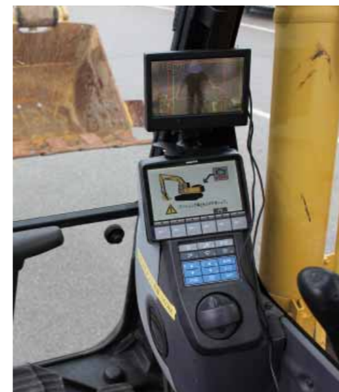
対象との距離を正確に計測するカメラを機械後方に設置。AIがセンサー内に入った対象を「人」と「物」に分けてモニターに表示、人と認識された場合に機械を強制停止する接触防止システム「ナクシデント」 A rear-mounted construction equipment camera for accurately measuring distance to physical objects. “AI” separates objects detected by the sensor into “people” and “objects” and displays them on a monitor; the Naccident “contact prevention system” forcibly stops the equipment when an object is recognized as a person
