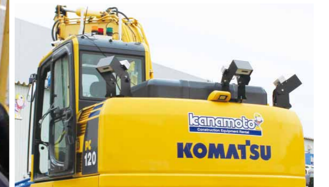
対象との距離を正確に計測するカメラを機械後方に設置。AIがセンサー内に入った対象を「人」と「物」に分けてモニターに表示、人と認識された場合に機械を強制停止する接触防止システム「ナクシデント」 A rear-mounted construction equipment camera for accurately measuring distance to physical objects. “AI” separates objects detected by the sensor into “people” and “objects” and displays them on a monitor; the Naccident “contact prevention system” forcibly stops the equipment when an object is recognized as a person
